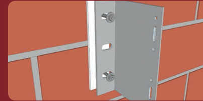
Securing angular support profiles to the wall consoles
