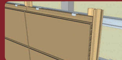
Installation of the top tile row
